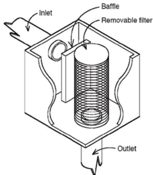
Figure 4.6-4. Roof Washer (TWRB, 2005).
