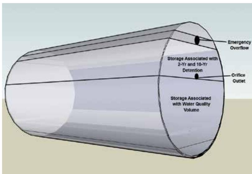
Figure 4.6-6. Tank Design 2: Storage Associated with SWTV, 2-year and 10-year Storms. (Source: Alex Foraste)
