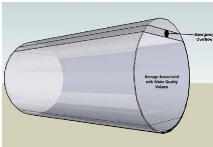
Figure 4.6-5. Tank Design 1: Storage Associated with the Design Storm Volume Only (Source: Alex Foraste)
