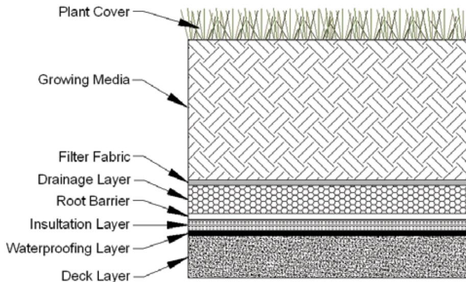
Figure 4.5-2 Green Roof Cross Section
