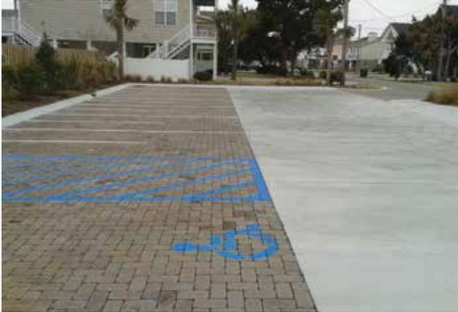
Figure 4.3-1. Permeable pavement parking spaces in North Myrtle Beach, SC (Photo: Travis DuPree)
