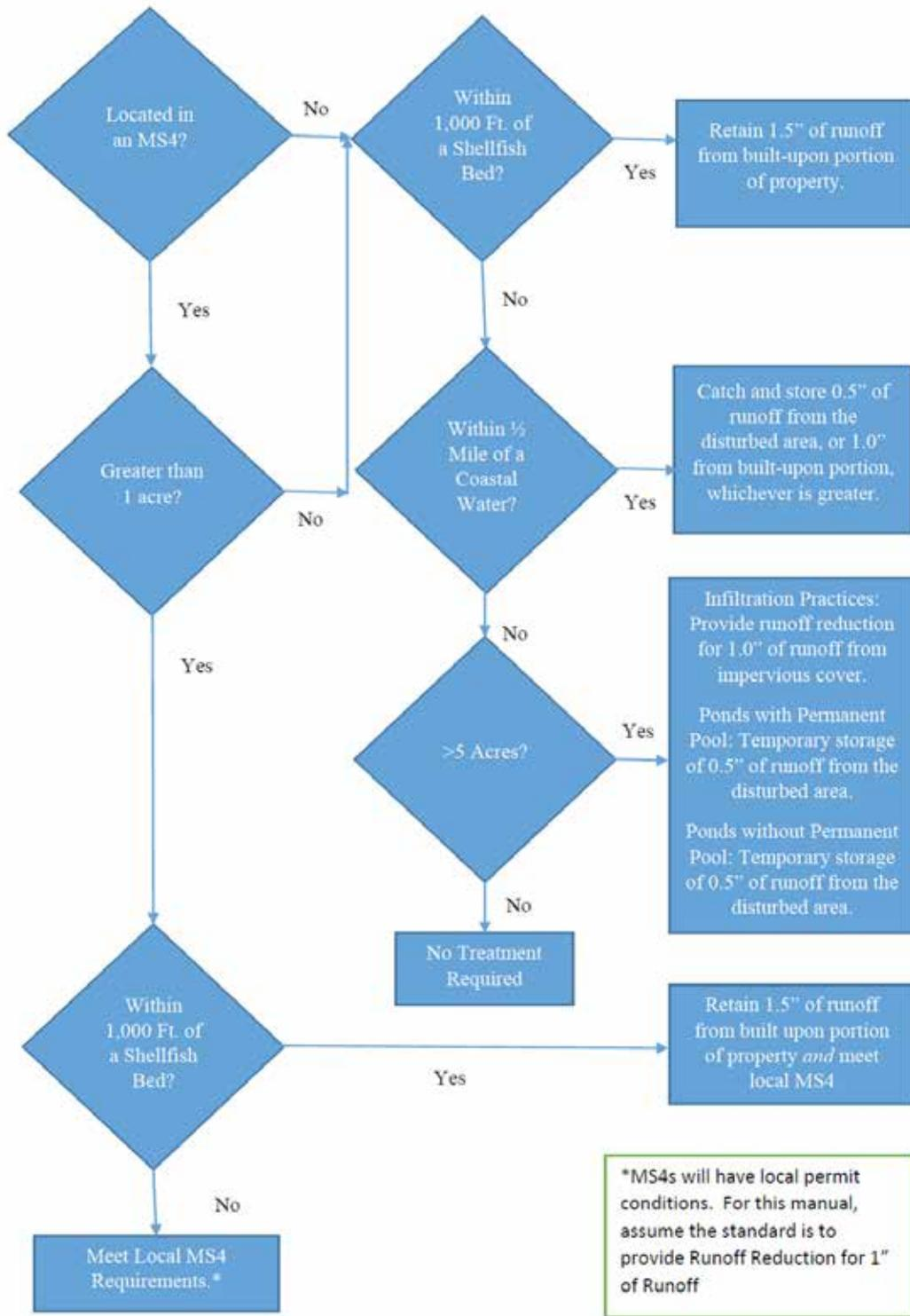
Figure 4.1-1. Flowchart to Determine Stormwater Management Requirements
